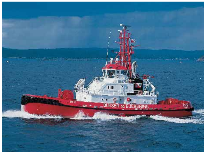
Figure 3.5 Bess – First "Skeg Forward" design of VSP Escort Tugboat
