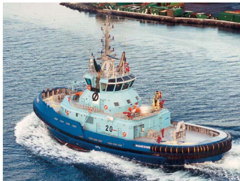
Figure 3.6 Ajax – VSP Escort Tug with bi-directional capability
