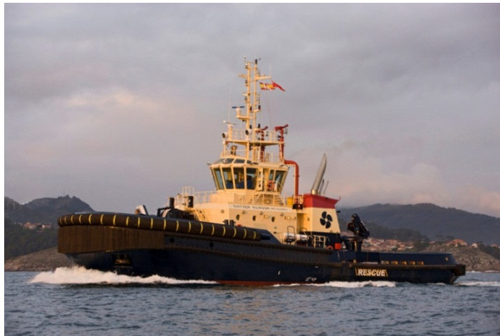
Figure 3.7 Svitzer Kilroom : 116 tonne BP ASD Escort Tug
