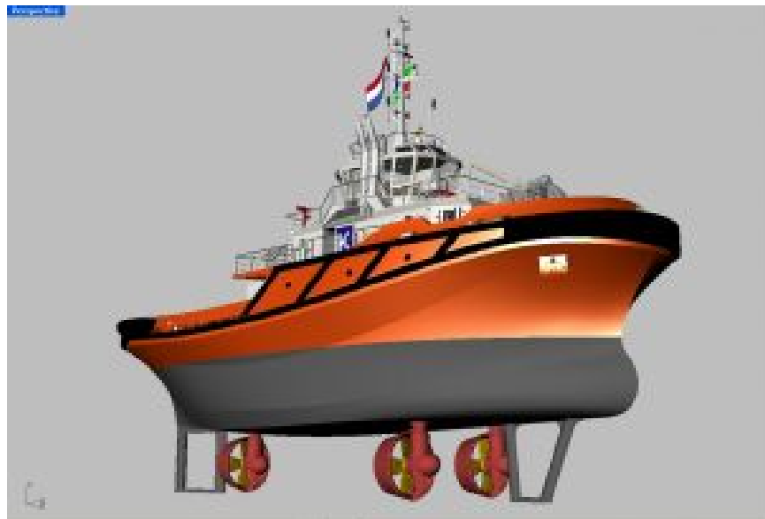
Figure 3.10 37 Metre Rotor Tug Configured as an Escort Tug (100 tonne BP)
